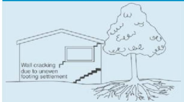
As the weather pattern changes and the soil begins to dry out, the external footings will be first affected, beginning with the locations where the sun's effect is strongest. This has the effect of lowering the external footings. The doming is accentuated and cracking reduces or disappears where it occurred because of dishing, but other cracks open up. The roof lines may become convex.
